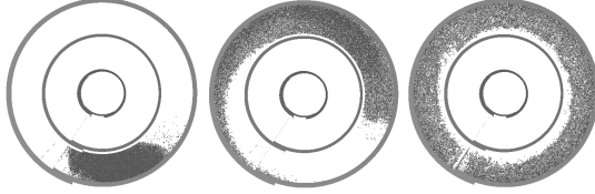
Fig. 5: Lunar regolith transport under 4.4 Hz frequency at: (L) t = 5 s; (M) t = 15 s; (R) t = 90 s (steady-state).
